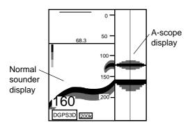
Figure 2-10 A-scope display plus normal sounder display
